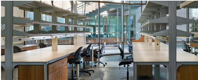
The single-story, 12,605-square-foot laboratory wing is home to 125 scientists and is where JCVI's most meaningful work happens. It includes wet bench research and dry research workspaces. The labs use an innovative "plug-and-play" casework system that allows researchers to modify spaces to suit their needs.
